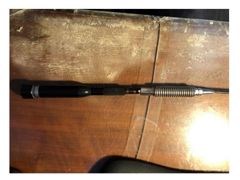
The finished project will look like this. Most of the straight springs I have looked at all had a one piece 3/8x24 stud on one end of the spring and a threaded hole on the other. Mounting the spring to the coil requires a 3/8x24 antenna mount nut.
