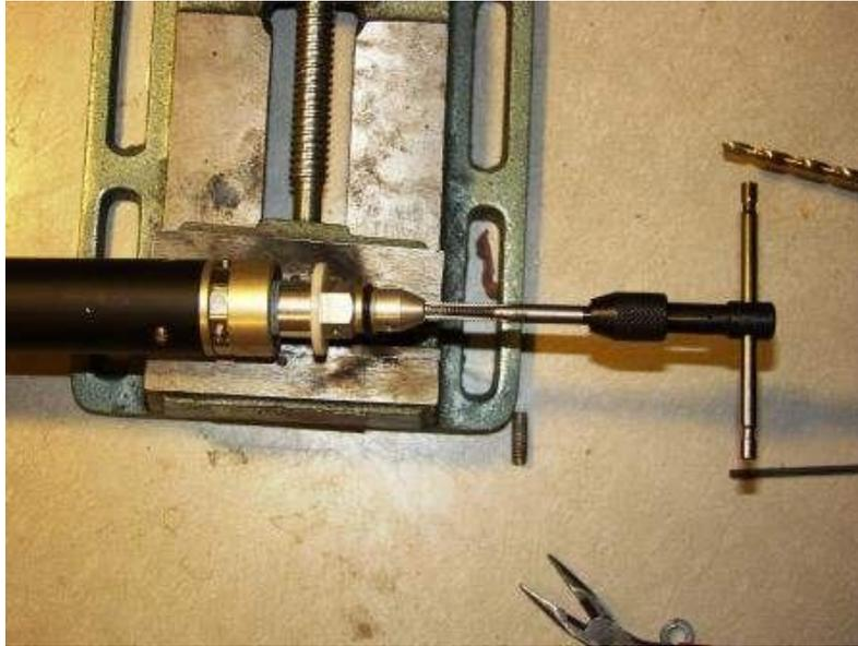
7. Install the stud 1/4 x 20 stud into the antenna coil before replacing the coil outer cover and weather boot.
