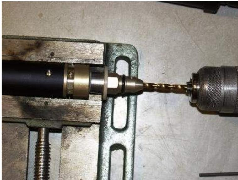
6. After drilling the hole, carefully tap the hole with a 1/4 x 20 SAE thread. I would personally recommend cutting only three or four threads at a time the backing out several turns to help clear the hole before cutting more threads.
