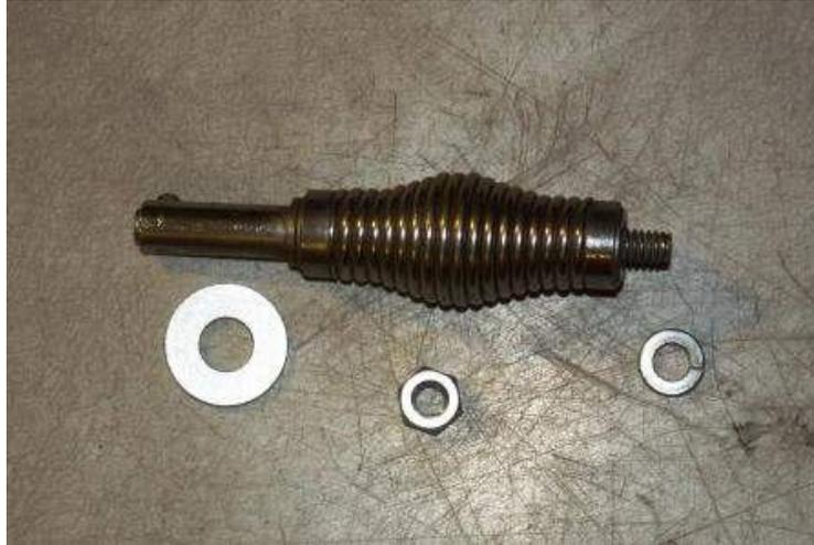
5. Enlarging the hole. When drilling out the center of the whip holder, be sure to secure the upper coil section to prevent rotary flex by the drill. Use a #7 drill bit. This is the recommended size bit for the 1/4x20 thread. A tap/bit combination can be purchased at Home Depot for about \$6.00. Be careful when drilling not to go too deep. I went only to below the set screw openings.
