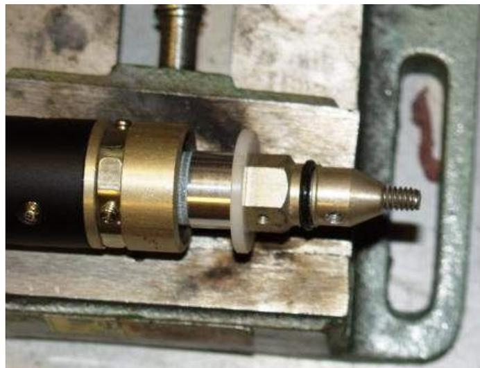
8. Slide the cover over the coil top section over the coil, install the set screws, and cut the nipple off the rubber rain boot with a razor blade. The final step is to screw the spring on the thread and tighten.
