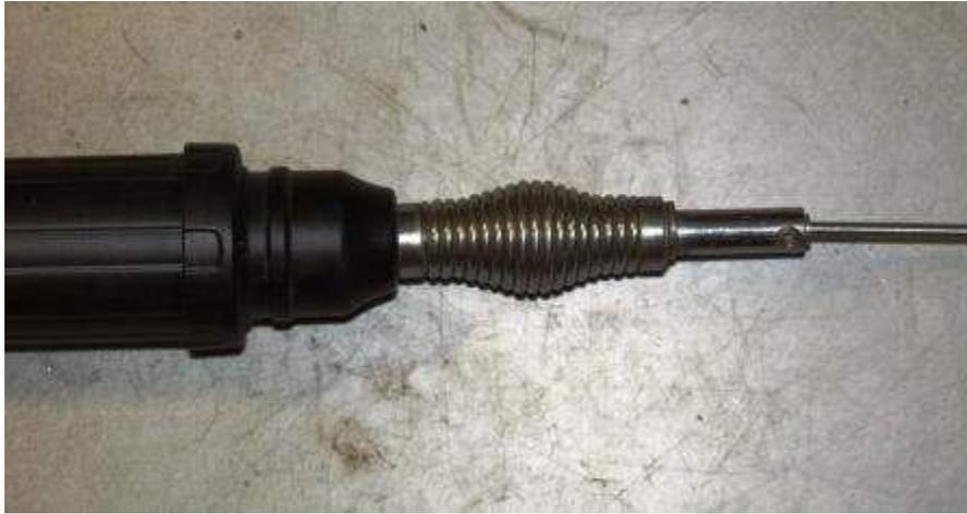
9. The following photos showing why the whip spring and base spring are so badly needed on the ATAS-120A.
